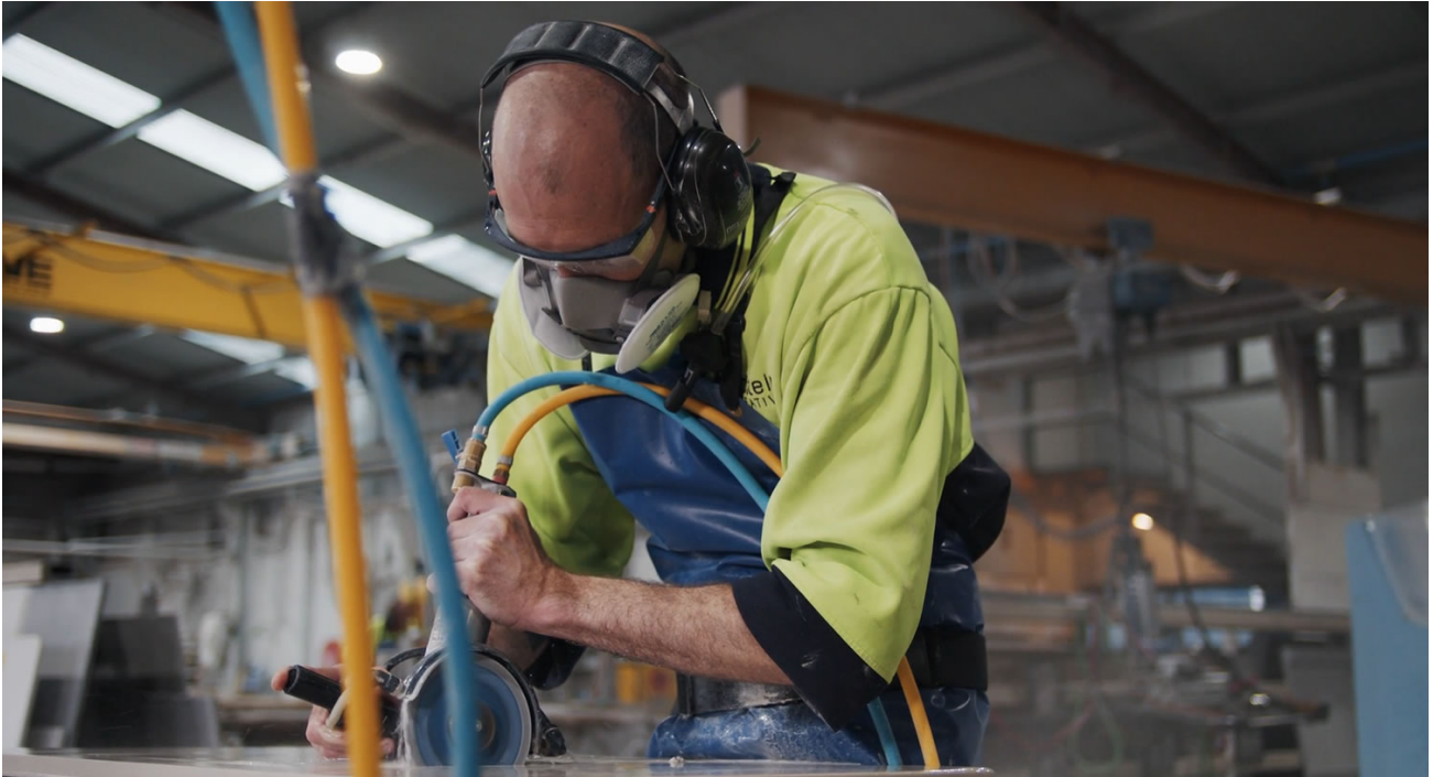
Image 5: An appropriate combination of controls may including wet cutting, respiratory protection and hearing protection.
